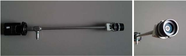
Fig. 2. Prototype 3D laparoscope with rotating polarizer.
