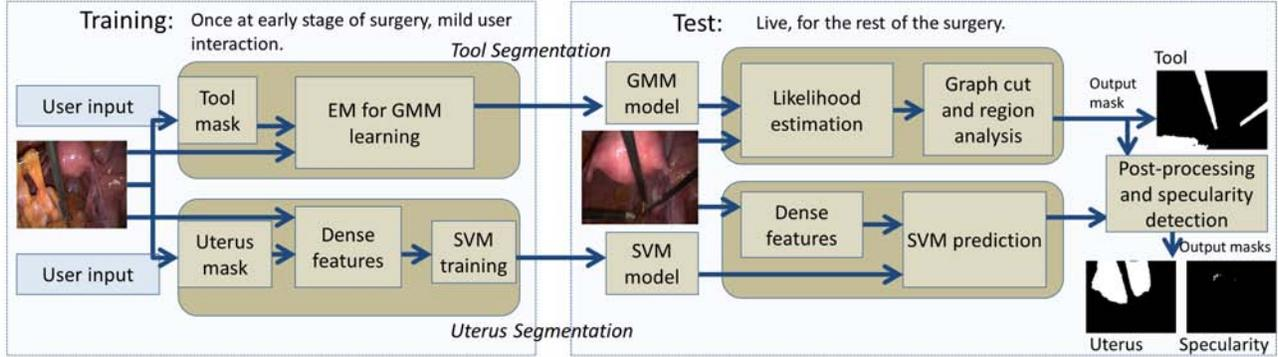
**Fig. 2:** A detailed process diagram of our four-class parsing. The actual processing is carried out after downsampling the input images for speed.
