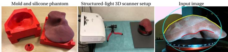
**Fig. 6** The silicone phantom’s mold, scanning setup and an input image with marked contours for testing the compared methods.
