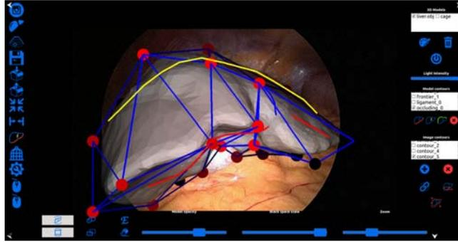
**Fig. 2.** Proposed Qt graphical interface: the left toolbar contains tools for loading the laparoscopic image and the preoperative 3D model, exporting and importing the entire scene, and generating the 3D cage; the right toolbar contains tools for managing the 3D model, image and model’s contours, and launching the registration; the bottom toolbar contains tools for zooming, editing the model’s transparency and shape.
