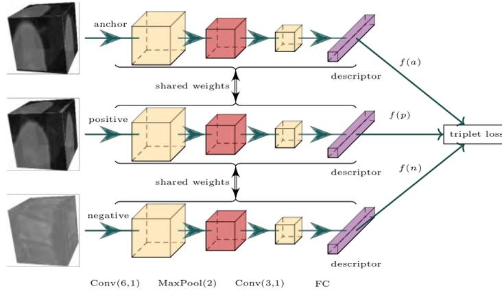
**Fig. 1.** Architecture of our CNN and the triplet-loss. The input patches are  $10^3$  voxels. The CNN has two convolutions with  $\tanh$  activation, one maxpooling and a fully-connected layer. The triplet  $\{a, p, n\}$  is passed through the network, and descriptor vectors are fed to the triplet loss.
