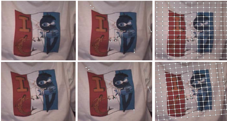
Figure 1: Registration of two images of a deforming Tshirt, shown top and bottom. (from left to right) Original images, the centres of the transformation and a grid mesh illustrating the mapping.
