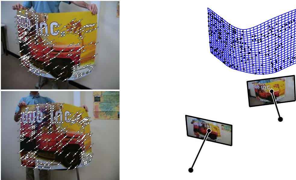
Figure 6.3: Paper (CVPR'07) – Generalized Thin-Plate Spline Warps . The two left images are ‘perspective images’ of a rigid smooth surface, overlaid with 206 point correspondences and epipolar lines. The right image shows the surface recovered through our RP-Warp.
