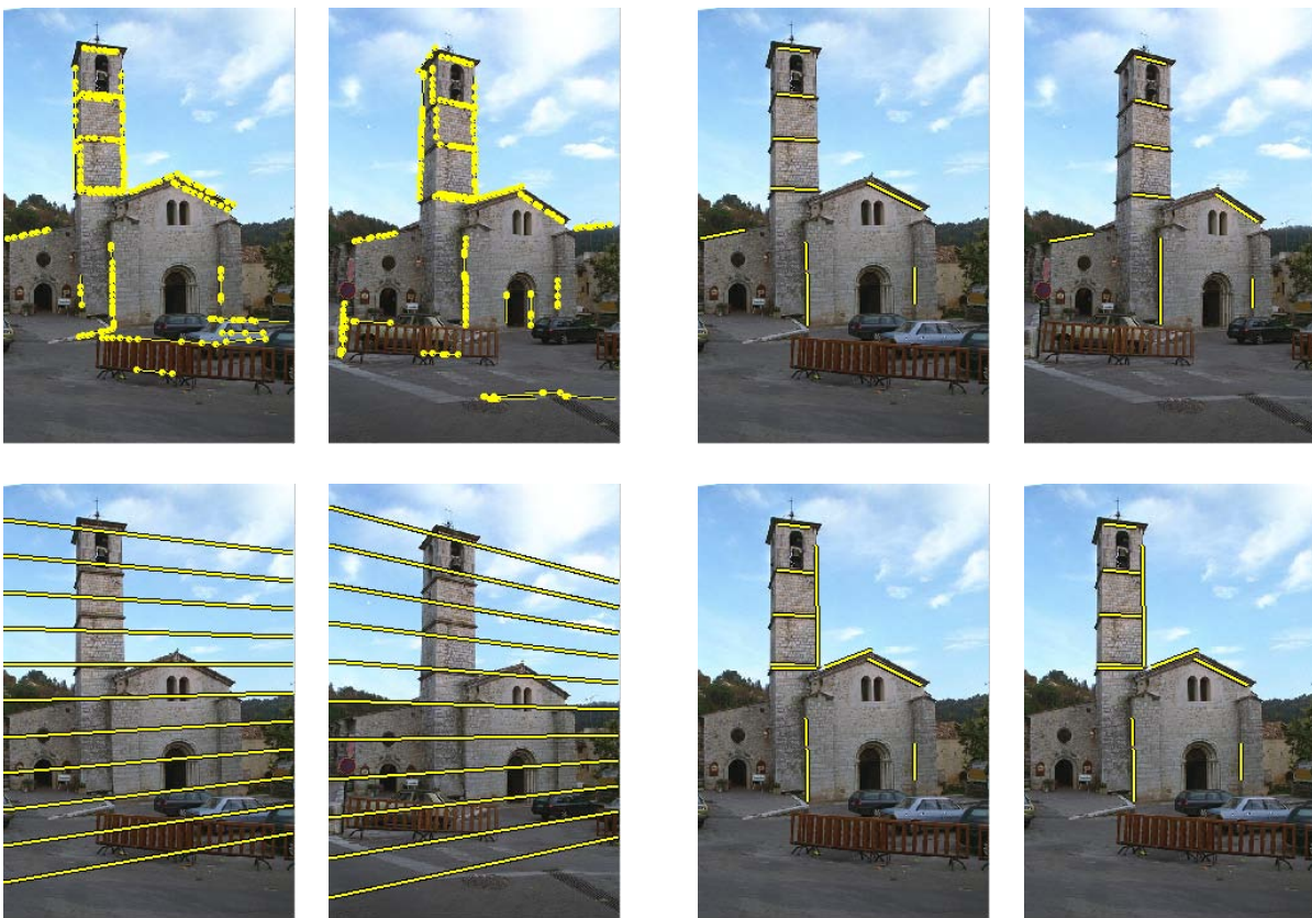
Figure 8.3: Paper (ECCV’04) – A Framework For Pencil-of-Points Structure-from-Motion . The images go by pairs. The top left image pair shows the detected POPs. The top right image pair shows the 9 putative matches we obtain. Here, there is no matching error. The bottom left image pair shows epipolar lines illustrating the estimated epipolar geometry. The bottom right image pair shows the 11 epipolar geometry guided matches we finally obtain.
