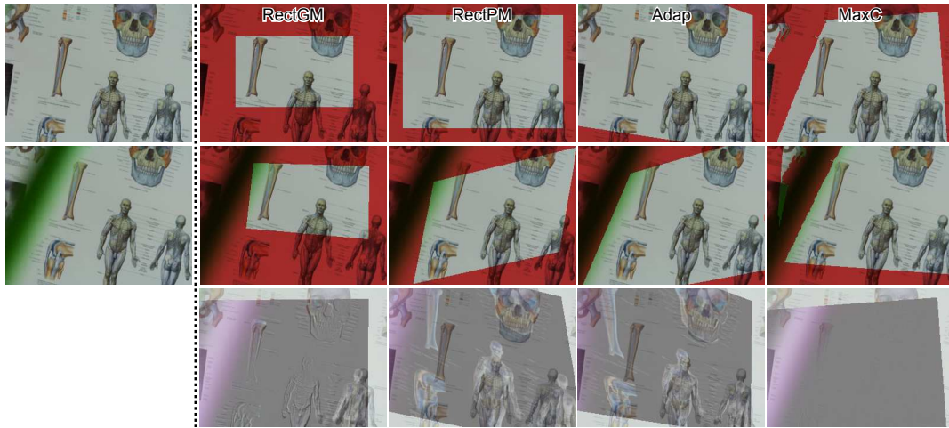
Figure 10: Examples of registration results for different algorithms. The first row corresponds to the source image, the second row to the target image, and the last row to the difference between the source and the warped target image. The red pixels are the pixels not included in the ROI during the last iteration of the algorithms. Note that the ROI computed by our approach (MAXC) corresponds to the true overlap (taking into account both the field of view and the occluder). Our approach is the only one that successfully registers this pair of images.
