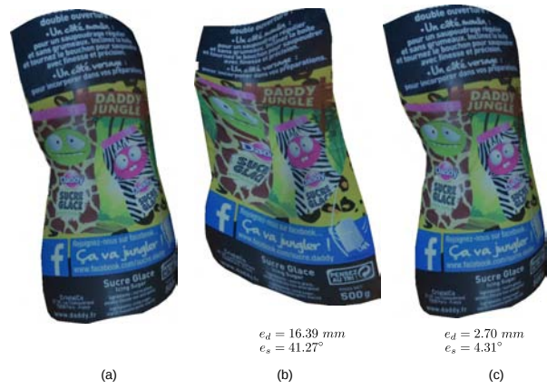
Fig. II: Results: (a) ground truth (b) typeII-P reconstruction with standard registration (c) typeII-P reconstruction with robust registration.
