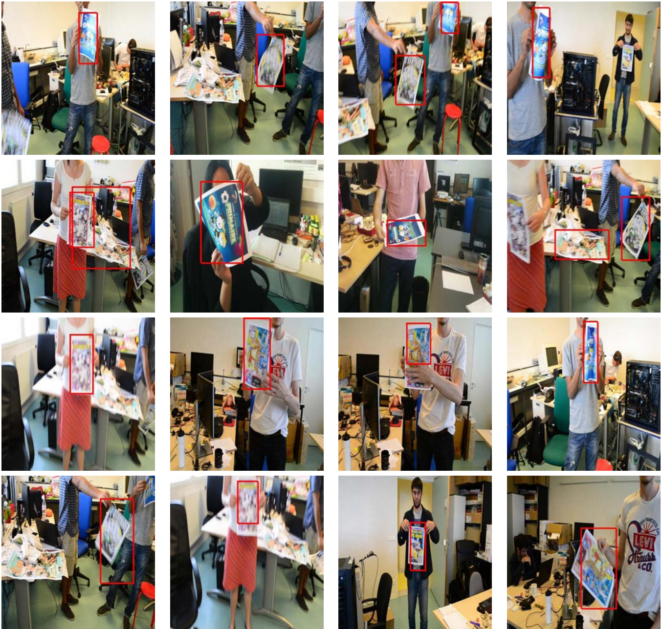
Figure 12: Selected examples of true positives on real images. The first image in the top row indicates that CNNs can cope naturally with lightings. The second image in the same row has a combination of motion blur and deformations. But the model still detects it.
