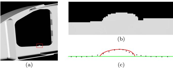
Fig. 6. RECONSTRUCTION OF A NONCONFORMITY BASED ON A SERIES OF VIRTUAL IMAGES OF AN OBJECT WITH AN ANOMALY. THE OBJECT IS SHOWN IN (A), WITH A CLOSE-UP IN (B). THE RESULT OF THE RECONSTRUCTION AROUND THE ANOMALY IS SHOWN IN (C), WITH THE ORIGINAL CURVE BEING A STRAIGHT LINE AND THE RECONSTRUCTED POINTS MATCHING THE ANOMALY IN BLACK.
