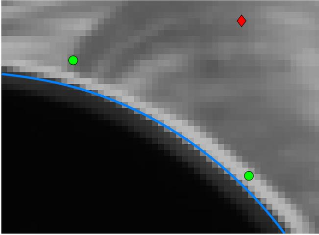
Fig. 5. A DETAIL, SHOWING THE CURVE BETWEEN TWO SIMILAR CONTOURS, THE PARALLEL MODEL CURVE TO THE LOWER LEFT AND A FALSE EDGE CAUSED BY SPECULARITIES TO THE UPPER RIGHT.
